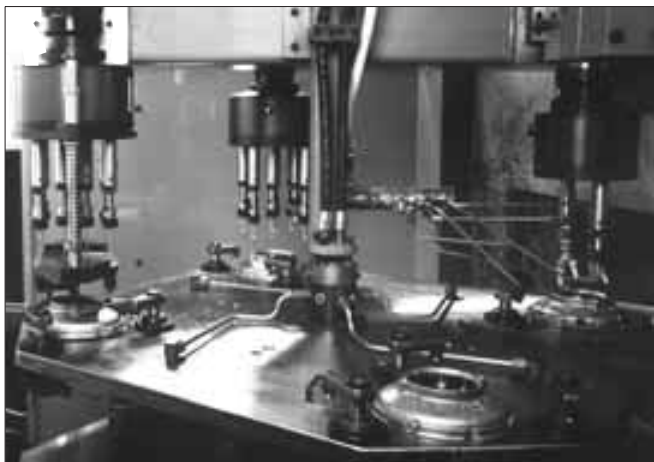
Rotary valve coupling with 8 stations for single-acting swing clamps. Application in a multiple-spindle machine with four stations for machining of aluminium covers. The four not required ports of the rotary valve coupling are plugged.
