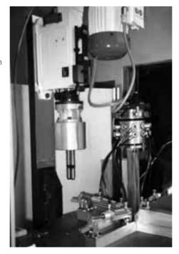
The figure shows the application of four station rotary indexing machine. In three operating stations the workpieces are bored by multiple spindle heads and threads are cut. At the load and unload station the machined workpieces are exchanged with unmachined ones. The pneumatic clamping elements are double-acting. The control is designed according to the circuit example on the next page; however every second port is not used.
