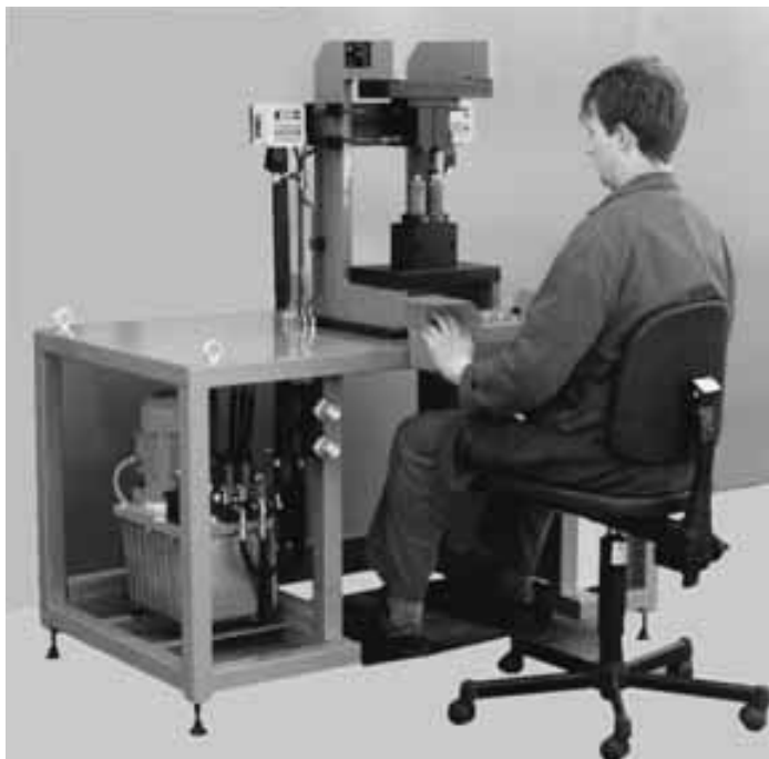
Stationary press-in frame for assembly, 20 kN version integrated with assembly sitting working place, hydraulic tandem cylinder and press-in force control. Application in the automotive supply industry: Assembly of bushings in valve rods.
