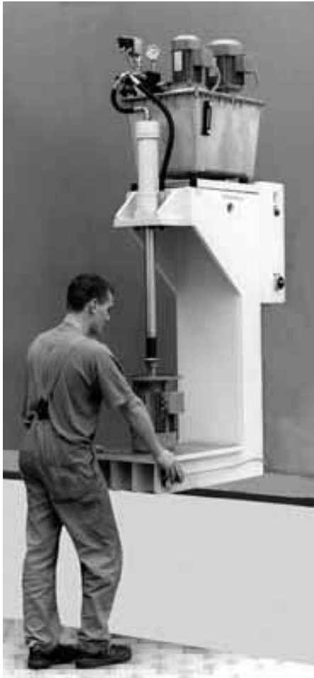
Stationary press-in frame for assembly, 50 kN version in solid welding construction with rapid and creep speed control of the hydraulic cylinder. Application in the gear industry: assembly of gear motors
