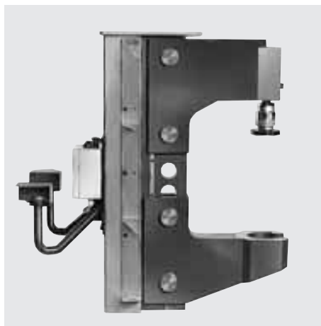
Mobile press-in frame for assembly, 80 kN version with opened lower contact piece for shafts. Application in the gear industry: Assembly of gears with one-part gear housings.
