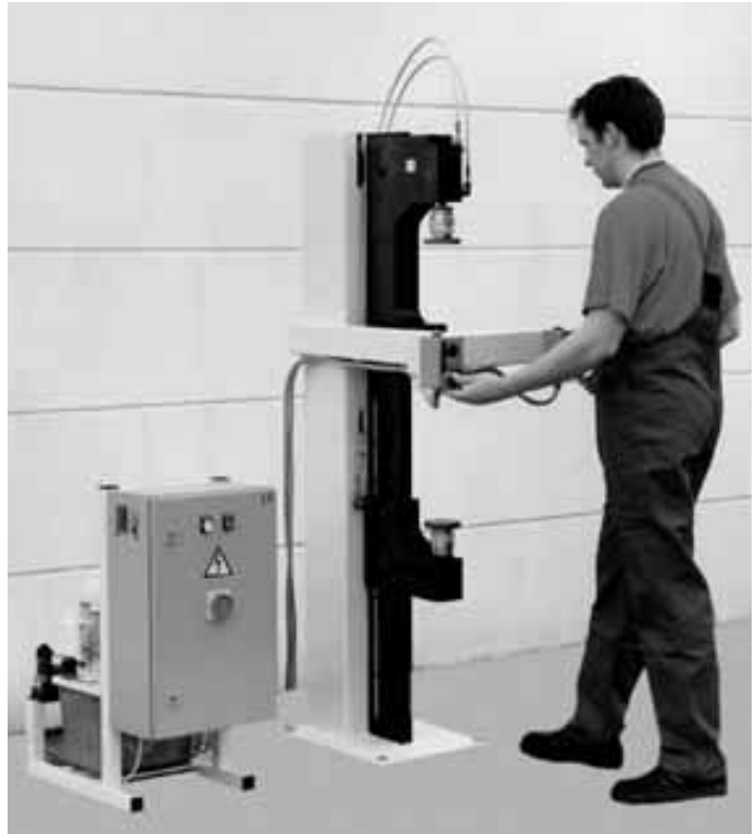
Stationary press-in frame for assembly, 63 kN version as stand-alone assembly fixture. Application in the automotive supply industry: assembly of cardan shafts
