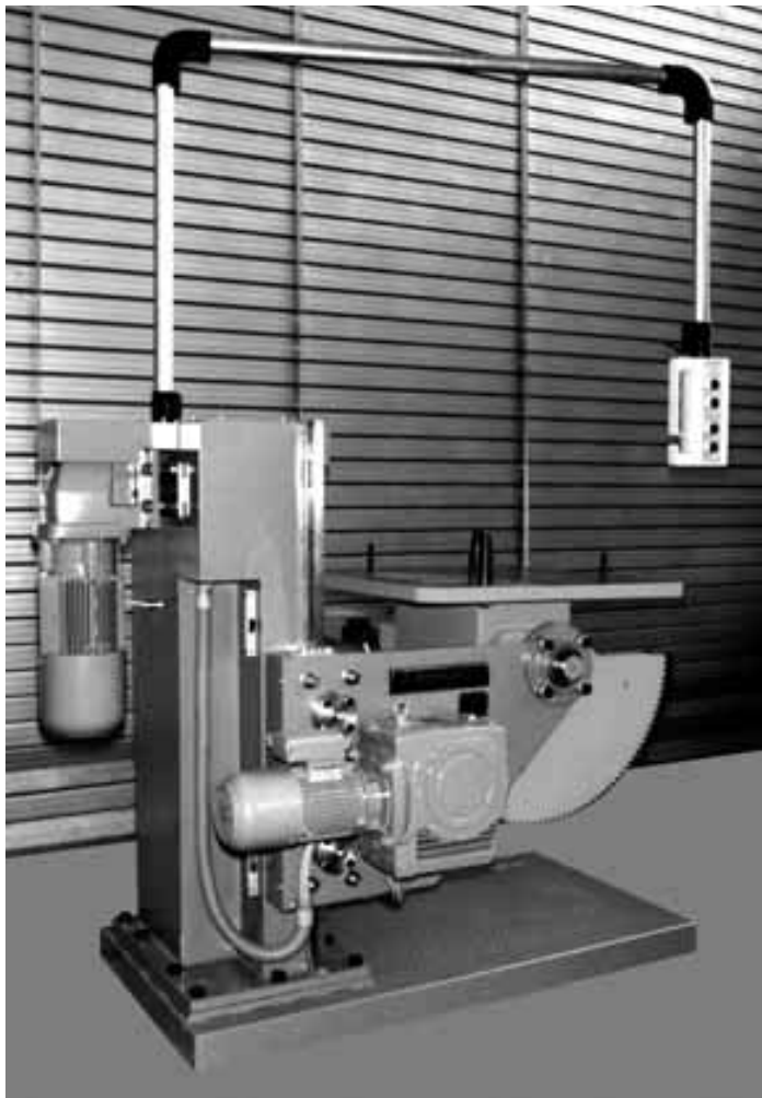
The figure shows a height-adjustable assembly table with rotating and tilting clamping surface in off-position
