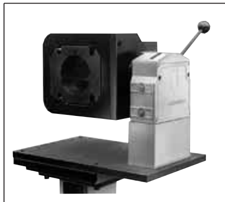
The above fixture consists of swivel element, spacer block, angle bracket and base plate.
