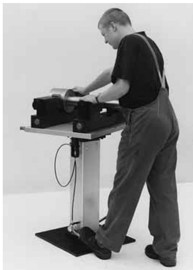
Concentric vice in preparation for machining of workpieces
