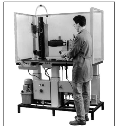
Height-adjustable assembly working place mounted on 3 electrically-operated lifting units.
